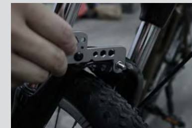
Hardened martensitic stainless steel 420
